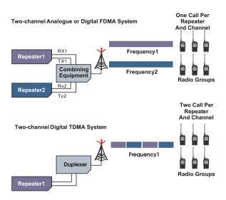
FDMA requires a dedicated repeater for each channel, plus expensive combining equipment to enable multiple frequencies to share a single base-station antenna. It can be particularly expensive to make combining equipment work with 6.25kHz signals, and there's typically a loss in signal quality and range when it's used in this way.
