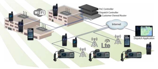
The PoC devices on the nationwide 4G/5G/LTE network use SIM cards to access the mobile operator's cellular network with an Access Point Name (APN) that routes the data traffic to the mobile operator's internet gateway. The PoC controller accesses the internet through the customer's network router.
